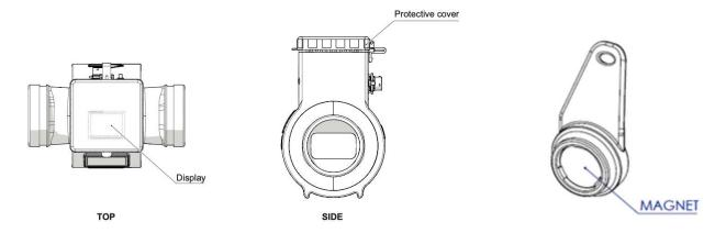
The MUT 7000 meter is equipped with a magnet for magnetic reed operation.
